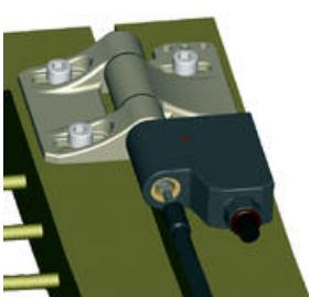
4. The bolt is tightened until the red indication disk between the hinge and switch unit is replaced with a green indication disk. Secure with extra 2 Nm (+10 %). Safety hinge is now operational and the contacts open while the door is opened.
