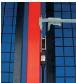
The hinge can also be installed between the door and the frame, in which case the hinge is mechanically protected. Installation width 20 mm, safety distance 120 mm.
