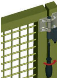
3. Tighten the special bolt located in the switch unit. Special torx head required for the setup is included in the delivery.
